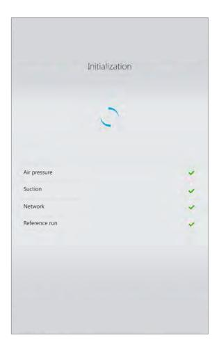
After checking the flap status and the compressed air supply, the device automatically performs several self-test steps (air pressure, filter status, network; it performs a reference run to position the axes).
