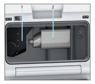
6. Swivel the milling arm (B axis)
