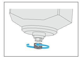
5. Clean the internal cones of the spindle with the cleaning cone from the spindle service set.
