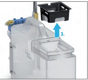
3. Fill the tank up to the fill level "max." (15 l) with tap water and PrograMill Fluid coolant concentrate (mixing ratio 7%).
