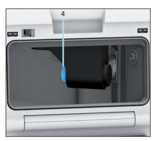
9. Swivel the milling arm to the starting position (B axis)
