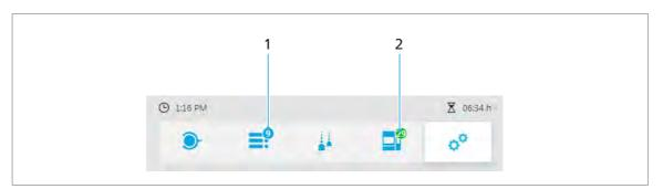
Messages (1) refer to situations that require the intervention of the user, but which are not critical for the system and the milling procedure (inserting tools, ejecting completed milling jobs, etc.).
