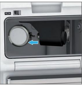
**3.** Insert the disc or block holder as illustrated in the milling arm.
