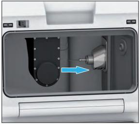
7. Clean the left side of the milling arm (B axis, pos. (3))
