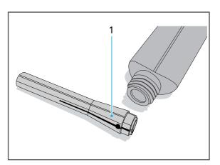
8. Screw the collet into the spindle until it stops using the screw-in piece.
