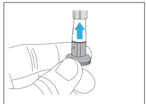
6. Clean the collet using the brush from the spindle service set, degrease it and make sure that the seals in the collet do not fall off.
